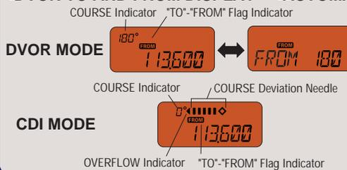
Press and Hold key 2 seconds to toggle the DVOR Radial Digits to the larger Display area.
